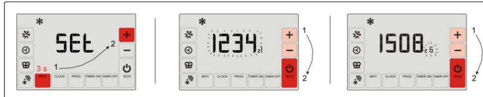
**NOTE:** The first time batteries are inserted, the configuration menu is directly accessed. Where configuration is not automatically accessed or where it is to be modified, enter SETUP mode (with the thermostat on) by pressing the combination of buttons shown in the figure. Then follow the same steps 1 to 4 as in the previous figure.
