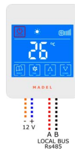
Fig. 16 ZEBRA thermostat connection diagram
